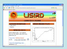
In spectrum mode, the user selects a wavelength interval and spectral resolution. The system gets the data from the various instruments and convolves it with the appropriate kernel.
